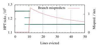
Figure 11: AM3358 cache channel, cache colouring. Cycle counter effect of mispredicts. N = 997, B = 1100 b/s.
