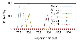
Figure 12: Response times for  $M_0$  and  $M_1$ . Shows peaks for OpenSSL 1.0.1c (VL), scheduled delay (SD) and 1.0.1e (CT), demonstrating reduced latency.  $10^6$  samples, binned at  $1\mu$ s.
